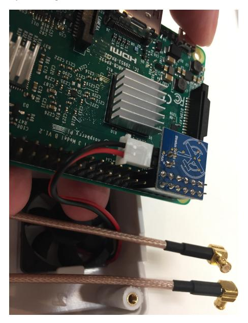
If you are not using the **AHRS board**, connect the fan to Pins 04 and 06, matching up the colors of the wires to those in the diagram:
