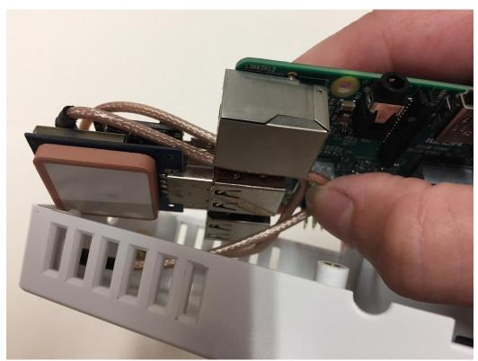
8. **Fasten the antenna pigtails** onto the case so that they are secure. **DO NOT** let one end of the pigtail rotate while tightening, this places strain on the cable and can twist the cable out of its connector. Use a wrench on **both ends** to tighten the nut. Make sure that it is secure enough to twist an antenna on and off, but not too tight that it cracks the case. Finish by situating the Raspberry Pi into the case.
