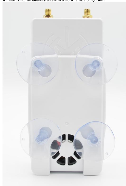
4. Slide the case in from above. Make sure that the fan faces towards the window. This will ensure that the GPS has a sufficient sky view.
